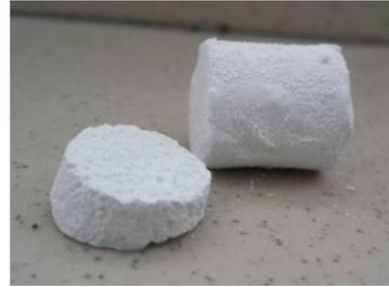
Fig 1. Gross image of a HA/TCP scaffold and its cross section after sintering
