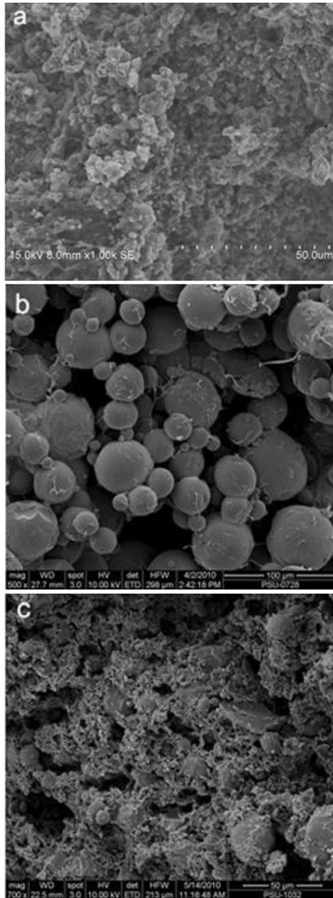
**Fig. 1:** The representative SEM images of scaffolds prepared by the compression molding/salt leaching technique (a); PCL microspheres (b); scaffolds prepared by the microsphere/chitosan cross-linking (c)
