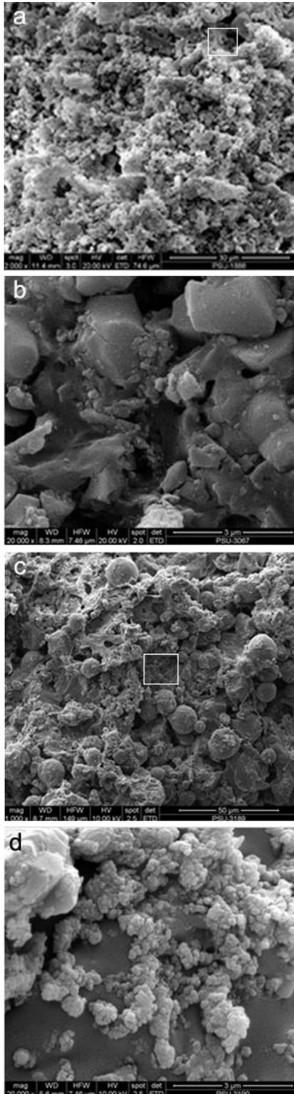
**Figure 3** Apatite layers formed on scaffold surfaces after immersed in PBS for 3 weeks: (a) “Sample 1”, (c) “Sample 2”, (b) and (d) the magnifications of (a) and (c), respectively; the corresponding un-immersed samples of (a) and (c) were respectively demonstrated in Figure 1a and 1c.
