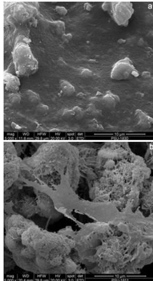
**Fig. 2:** The SEM micrographs of cell-seeded scaffolds cultured in the inducible medium for 5 days on "Sample 1" (a); and "Sample 2" (b)
